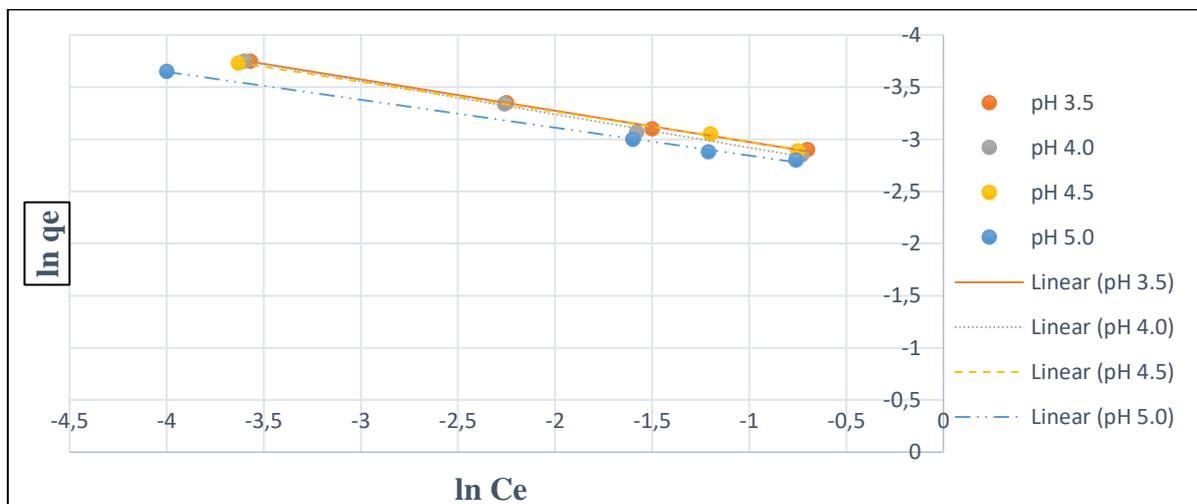
**Figure 11.** Freundlich isotherms at different pH levels for the removal of copper ions by keratin
