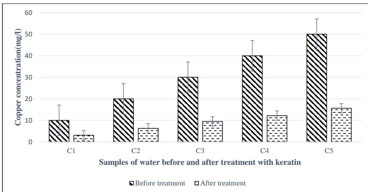
**Figure 13.** Concentration of Copper in the samples of water before and after addition of keratin
