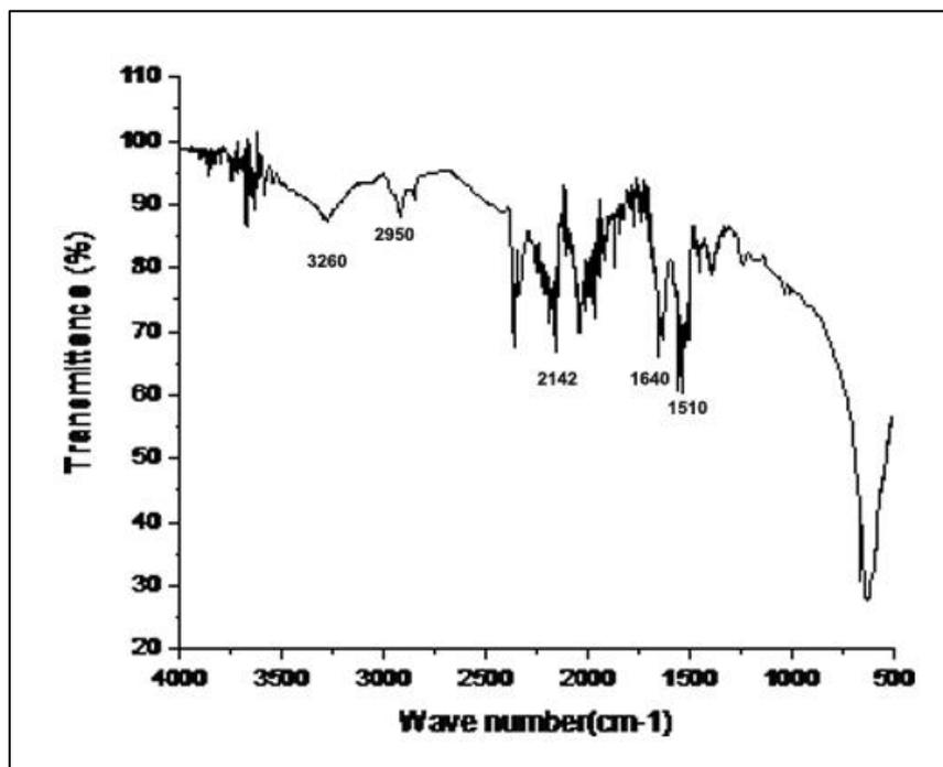
**Figure 2.** Peaks from FTIR data for extracted keratin protein
