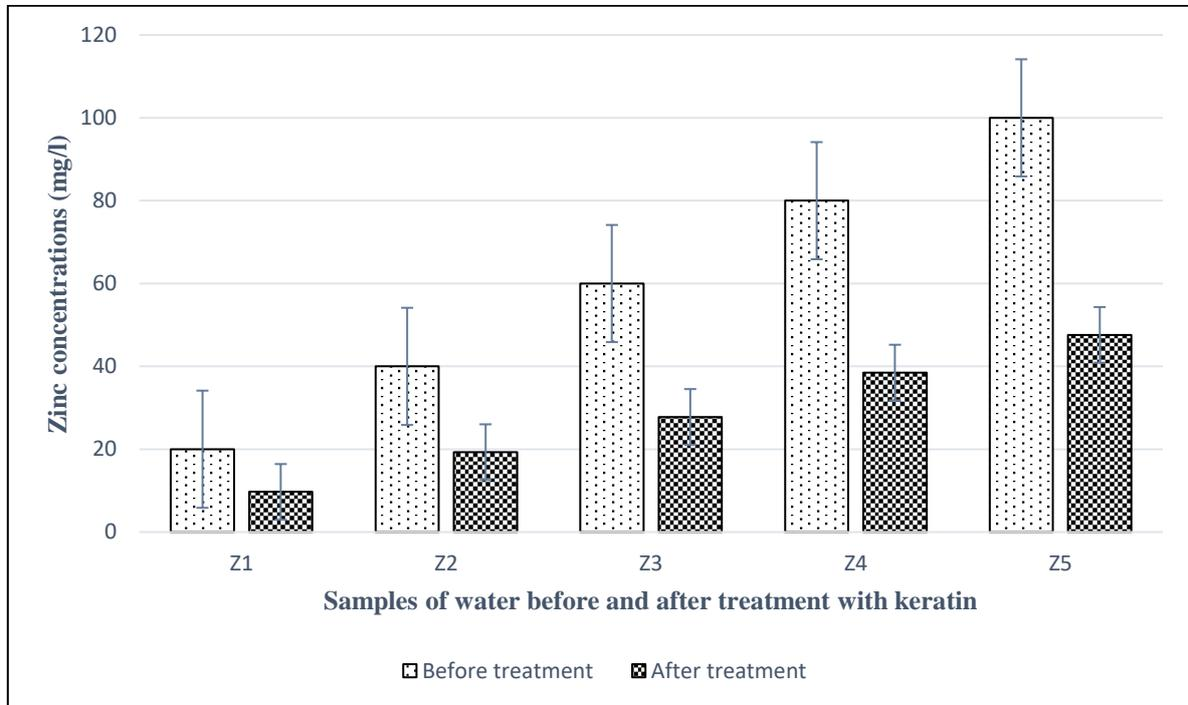
**Figure 12.** Concentration of Zinc in the samples of water before and after addition of keratin
