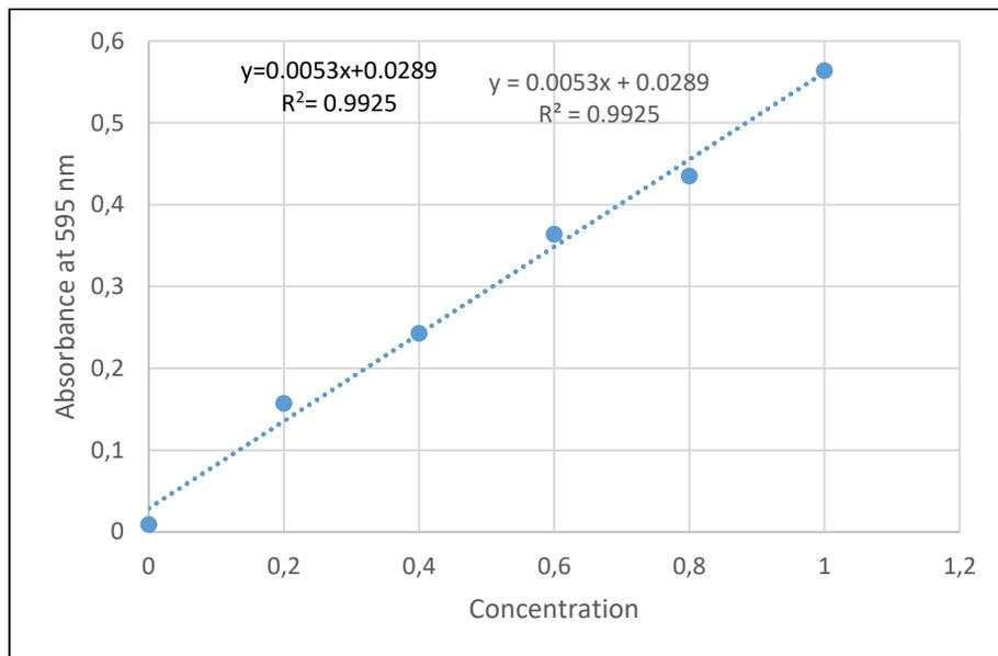
**Figure 1.** Standard curve for protein between concentration (mg/mL) and absorbance
