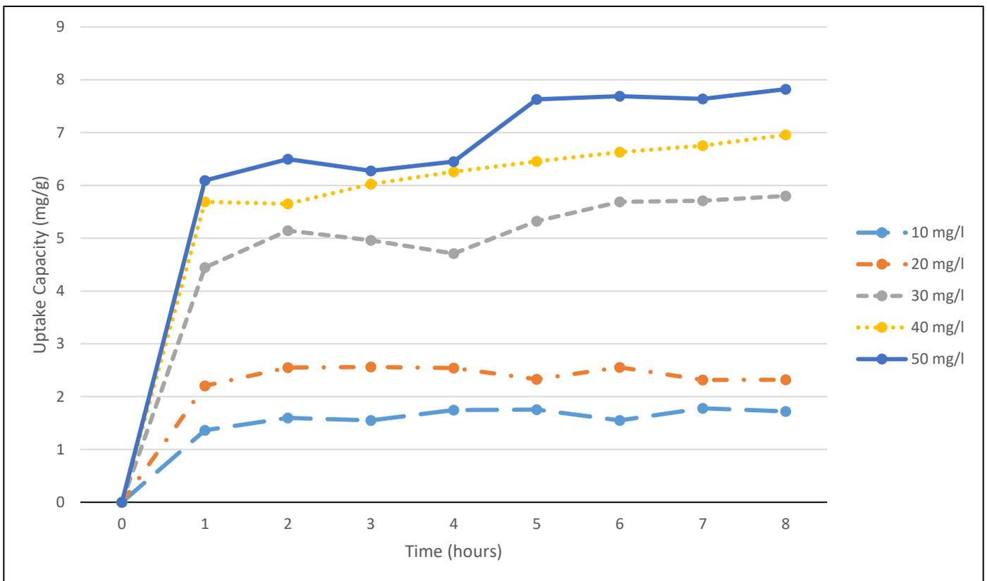
**Figure 6.** Uptake of copper ions at different initial concentrations (10-50 mg/L) by keratin adsorbent with its initial concentration of 5 mg/mL
