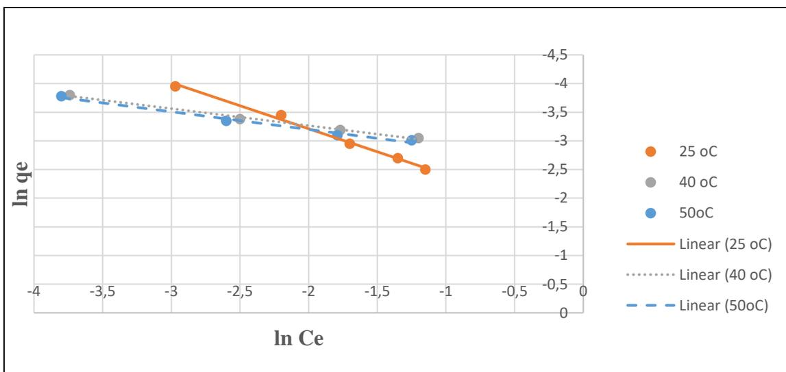
**Figure 9.** Freundlich isotherms for the removal of copper ions by keratin at temperatures 25, 40 and 50°C
