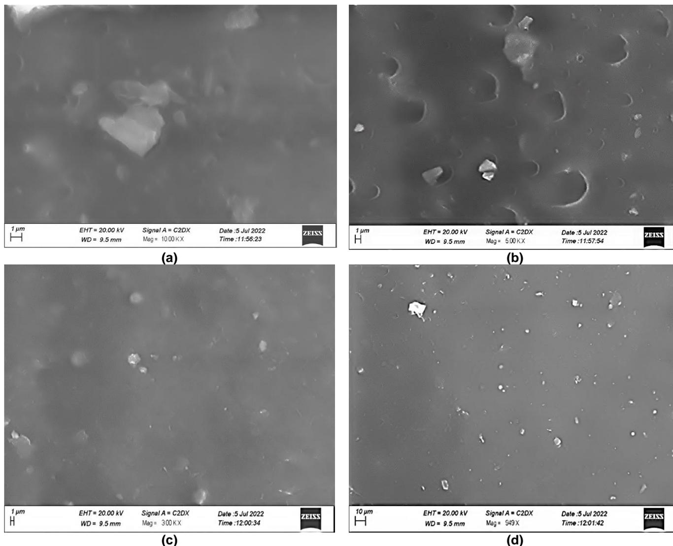
**Figure 4.** SEM showing keratin surface morphology with magnifications of **(a)** 10kx **(b)** 5kx **(c)** 3kx **(d)** 949x
