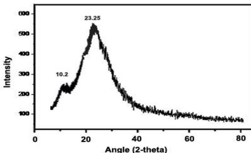
**Figure 3.** Angle and Intensity of keratin by X-Ray Diffraction (XRD)
