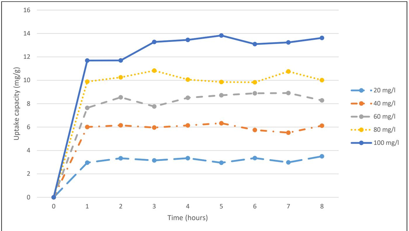
**Figure 5.** Uptake of zinc ions at different initial concentrations (20-100 mg/L) by keratin adsorbent with its initial concentration of 5 mg/mL
