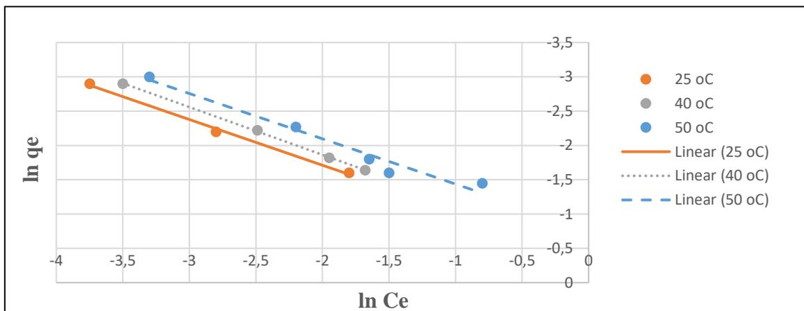
**Figure 8.** Freundlich isotherms for the removal of zinc ions by keratin at temperatures 25, 40 and 50 °C
