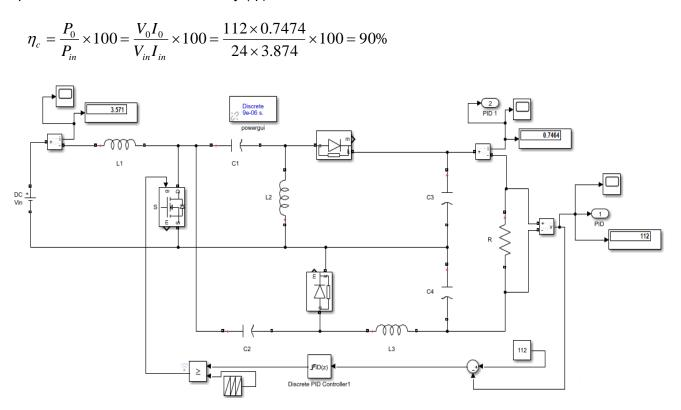
Figure 3. MATLAB / SIMULINK model of the proposed integrated DC-DC converter with PID controller
