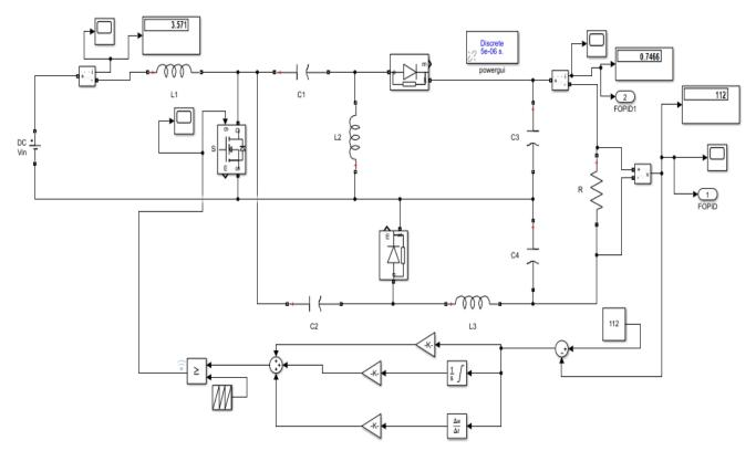
Figure 4. MATLAB / SIMULINK model of the proposed integrated DC-DC converter with FOPID controller
