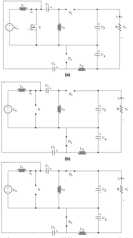
(C)Figure 2. Equivalent circuits of the suggested DC-DC converter -(a). Mode-I (b). Mode-II (c). Mode-III
