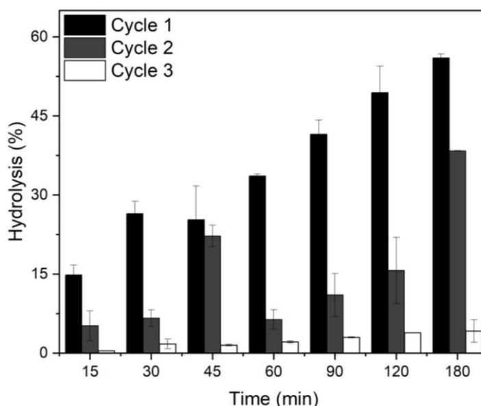
**Figure 4.** Enzymatic hydrolysis and recovery of Combi-Nb<sub>2</sub>O<sub>5</sub> through the conventional system.
