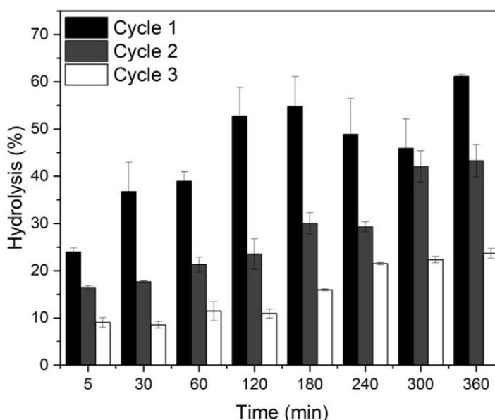
**Figure 5.** Enzymatic hydrolysis and recovery of Combi-PHB using the ultrasound system.
