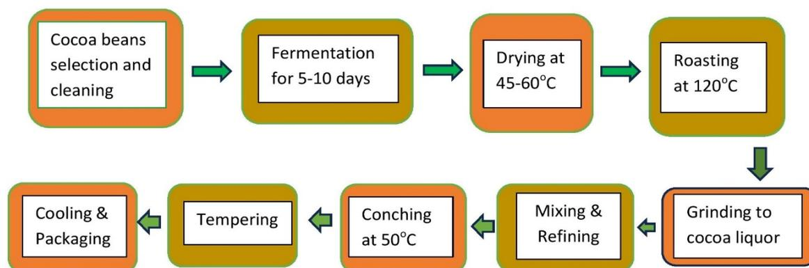
Figure 1. Cocoa processing for chocolate manufacture.
