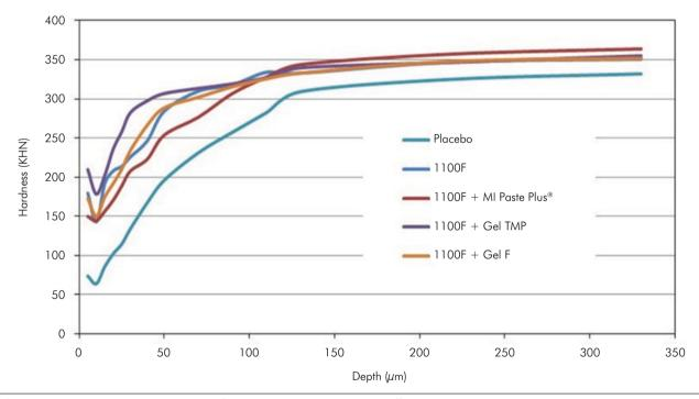
**Figure 1.** Cross-sectional hardness profiles (mean KHN, n = 12) at different depths (micrometers) in enamel blocks according to the treatments.
