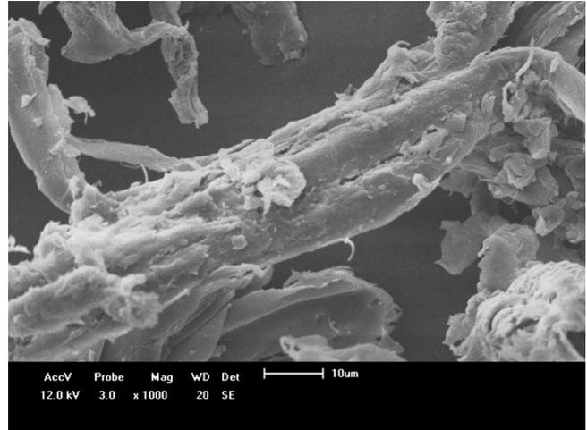
Figure 1: SEM micrograph of the fine wood dust waste.
