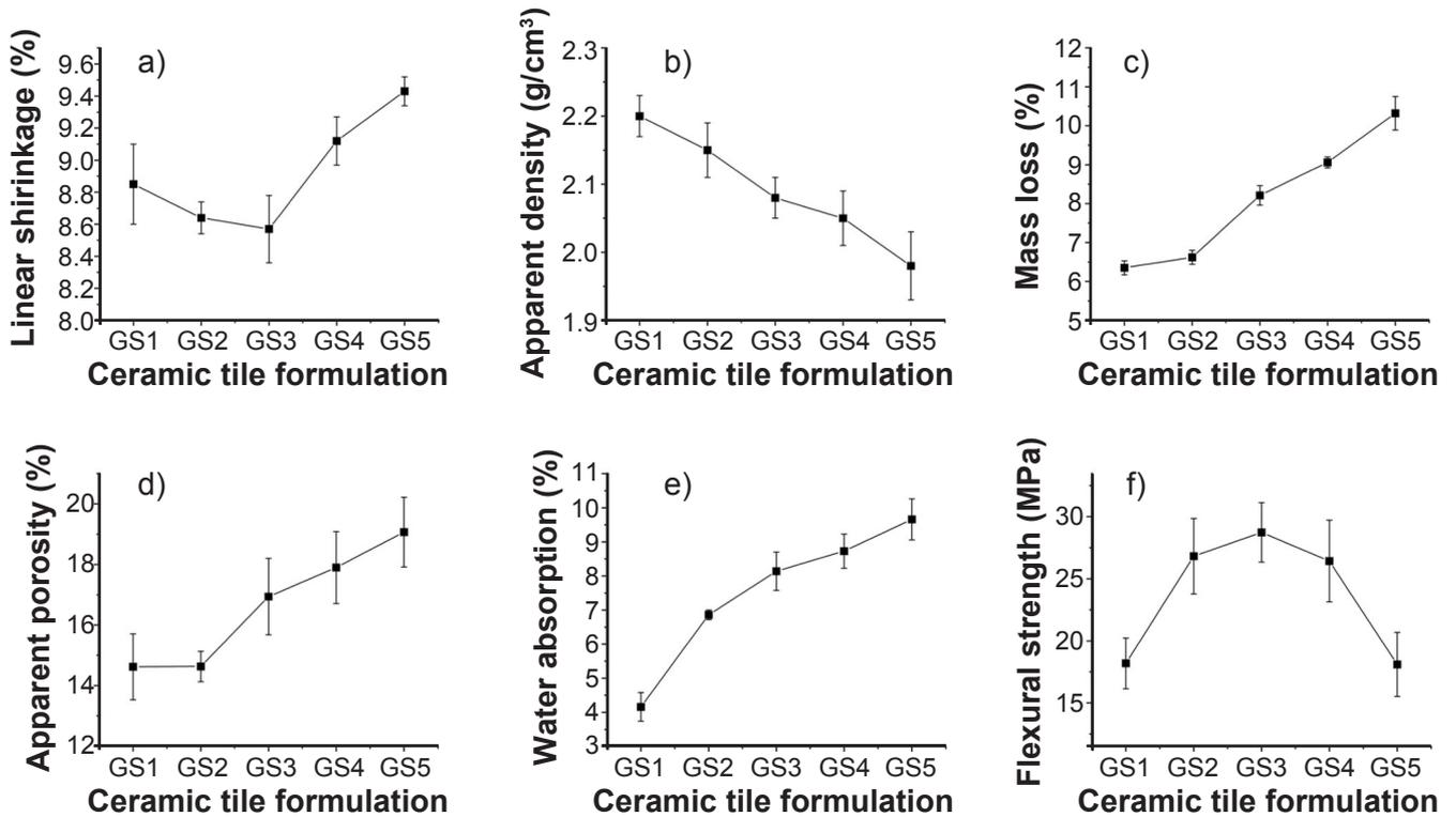
Figure 4: Technical properties of bi-layered ceramic tiles: a) linear shrinkage; b) apparent density; c) mass loss; d) apparent porosity; e) water absorption; and f) flexural strength.
