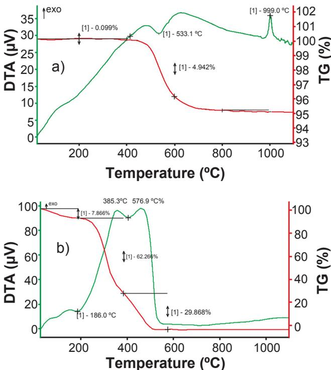
Figure 2: DTA/TG curves of: a) GBPO paste; and b) fine wood dust waste.
