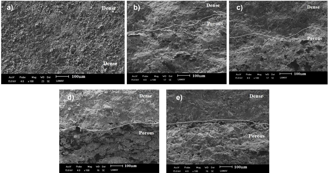
Figure 3: SEM micrographs of the fired bi-layered ceramic tiles: a) GS1; b) GS2; c) GS3; d) GS4; and e) GS5.
