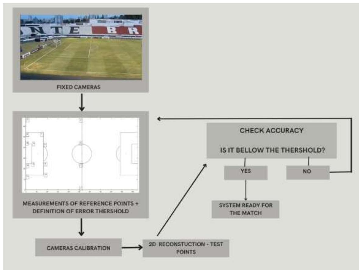
**Figure 1.** Workflow of the steps needed before the match starts for system calibration and accuracy evaluation during offside plays
