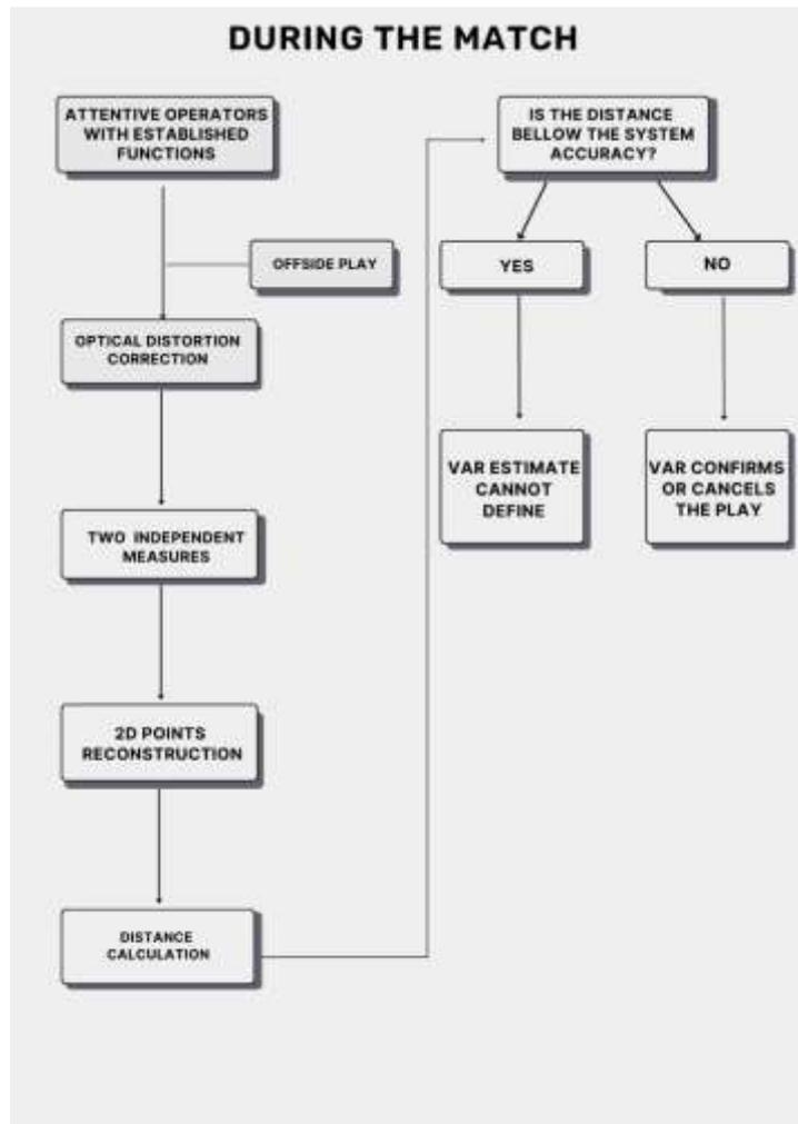
**Figure 2.** Workflow of the steps that is expected to be accomplished during the match by the VAR operators
