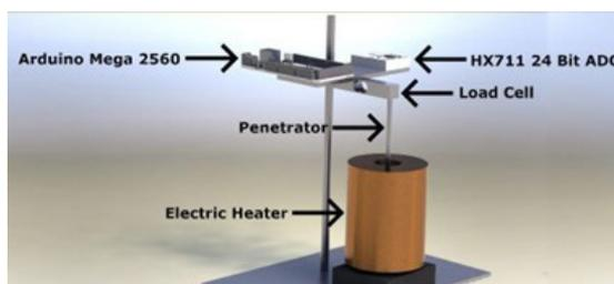
Figure 1. Schematic representation of prototype components.
