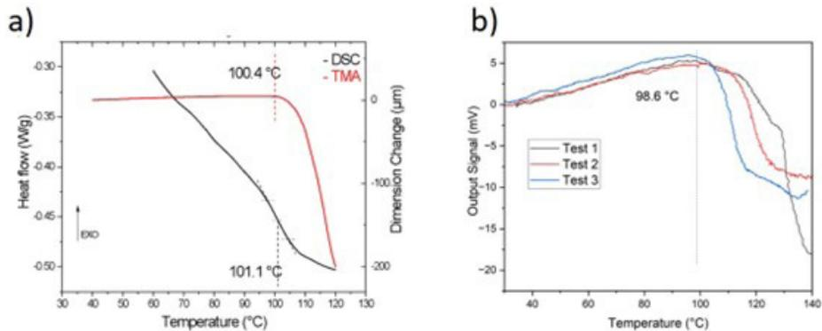
Figure 4. (a) DSC/TMA analysis of PS; (b) PS analysis by prototype (load cell-strain gauge).
