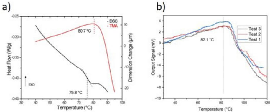
Figure 3. (a) DSC/TMA analysis of ABS; (b) ABS analysis by prototype (load cell-strain gauge).
