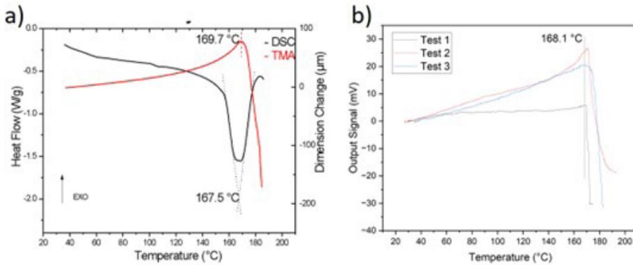
Figure 6. (a) DSC/TMA analysis of POM; (b) POM analysis by prototype (load cell-strain gauge).
