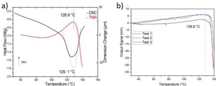
Figure 5. (a) DSC/TMA behavior for HDPE sample; (b) HDPE polymer behavior by prototype (load cell-strain gauge).
