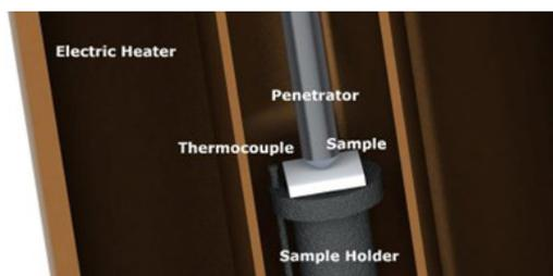
Figure 2. Cross-section view of the sample holder inside the electric heater.
