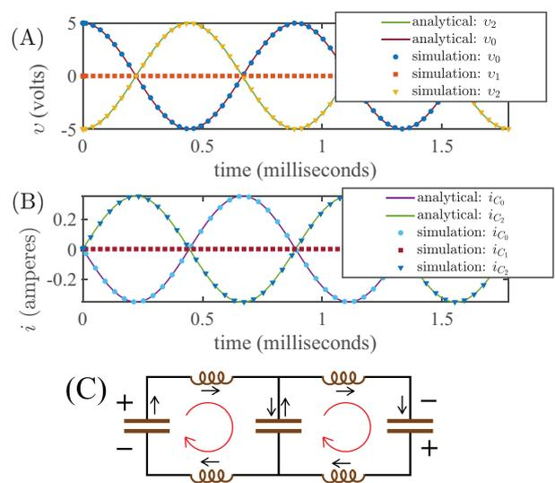
**Figure 2:** Slow mode in the two-loop circuit: (A) Voltage vs. time. (B) Current vs. time. (C) Current flow that is represented as  $\overrightarrow{0 \ 1 \ 2}$ .
