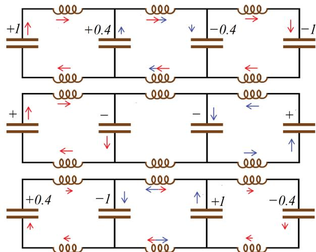
**Figure 9:** Current flows for  $N = 3$  loops. From top to bottom, the circuit is synchronized with the frequencies  $\omega_1$ ,  $\omega_2$ , and  $\omega_3$ , respectively.
