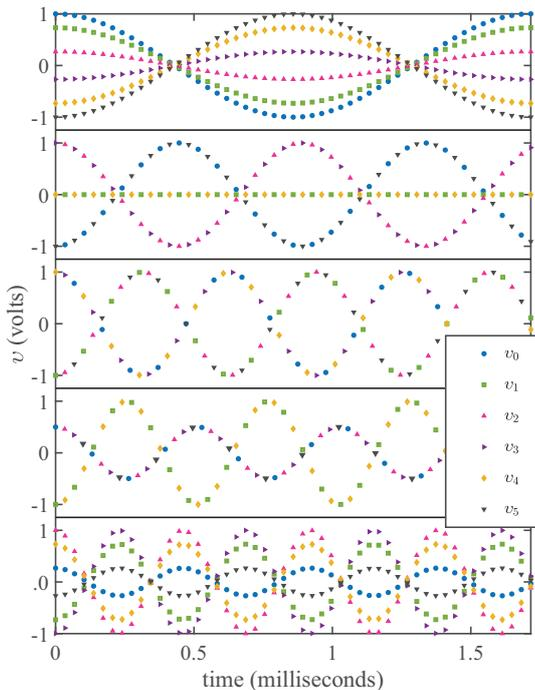
**Figure 11:** Voltages for an  $N = 5$  circuit. From top to bottom, one shows the results from the slowest to the fastest mode.
