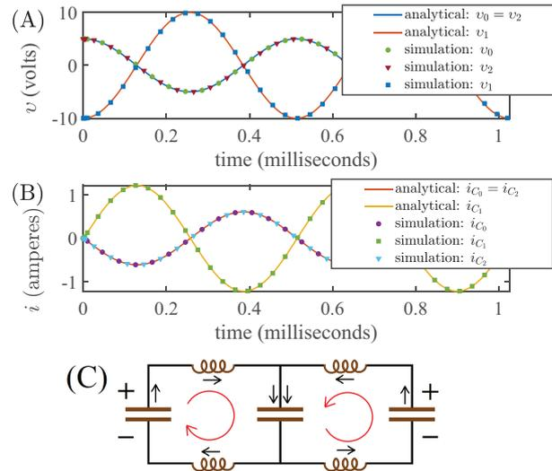
**Figure 3:** Fast mode in the two-loop circuit: (A) Voltage vs. time. (B) Current vs. time. (C) The current flow that can be illustrated as  $0 \ 1 \ 2$ .
