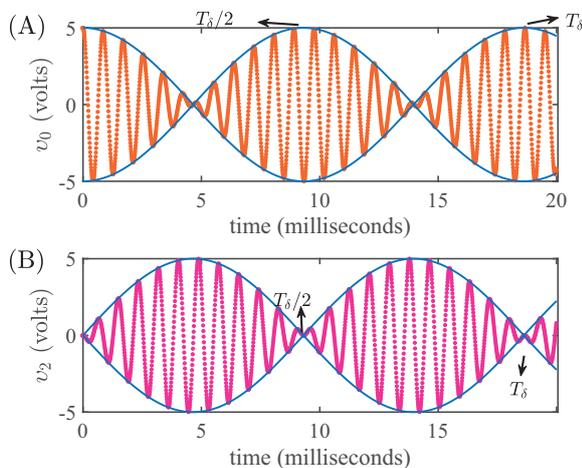
**Figure 5:** Two-loop circuit with beating patterns on the external capacitors.
