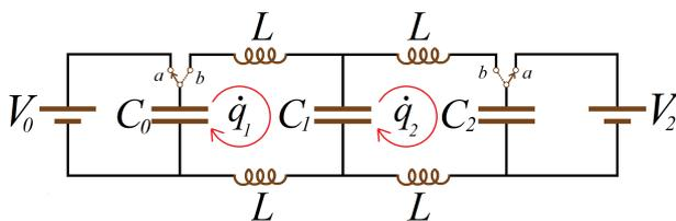
**Figure 1:** Two-loop circuit connected to the batteries for  $t < 0$ . At  $t = 0$  the switch changes from "a" to "b" and the oscillations begin.
