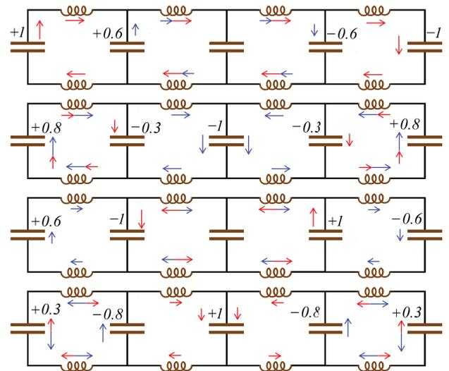
**Figure 10:** Currents flow in a system with  $N = 4$  loops. From top to bottom, the excited NFs are  $\omega_1$ ,  $\omega_2$ ,  $\omega_3$ , and  $\omega_4$ .
