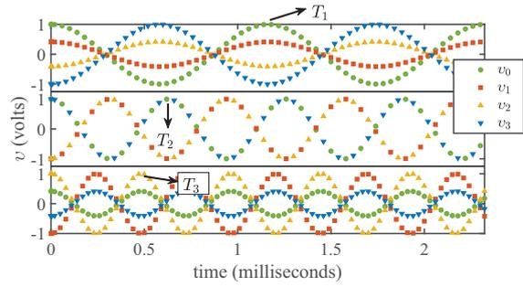
**Figure 8:** Normal modes oscillations for  $N = 3$ . From top to bottom: voltage on the capacitor for the slow, intermediate, and fast modes.
