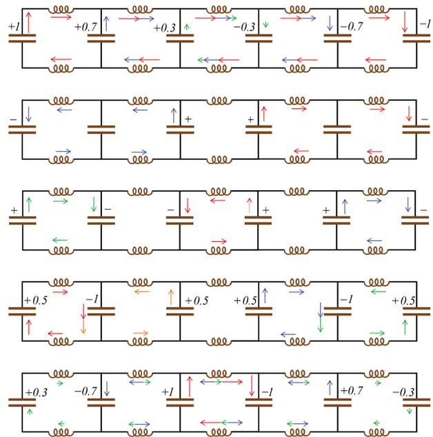
**Figure 12:** Currents flow in a system with  $N = 5$  loops. From top to bottom the natural frequency  $\omega_1, \omega_2, \omega_3, \omega_4,$  and  $\omega_5$  was excited.
