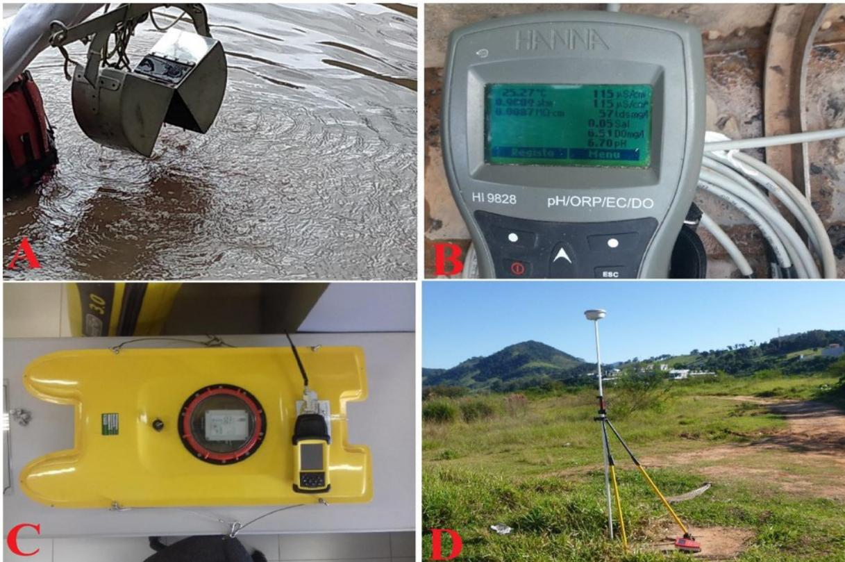
**Figure 3.** Equipment used in fieldwork: (A) Van Veen type sampler; (B) Hanna HI9828 multiparameter probe; (C) Qliner V3 and flow meter; (D) Leica LI and L2 GNSS receiver.
