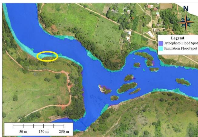
Figure 19. Orthophoto from the period January 2022 with comparisons of the flood spots generated by the orthophoto taken during the event and by the 2D hydrodynamic simulation.
