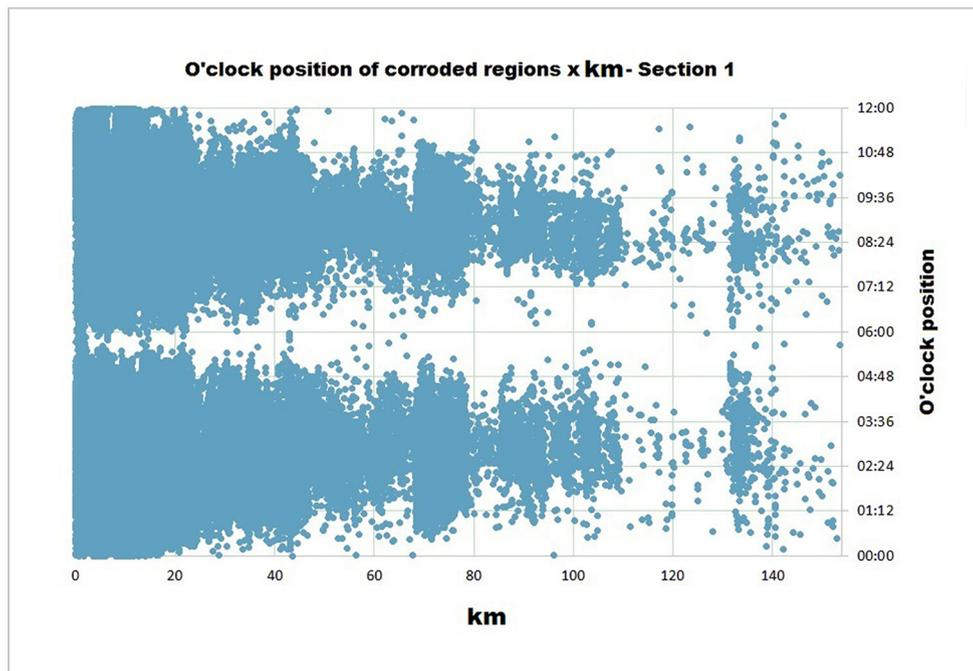
Figure 8 - O'clock positions of corroded regions along the length of the pipeline - Section 1.
