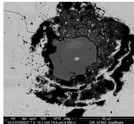
Figure 5 - Pore partially filled with aggregate and containing a calcite grain.
