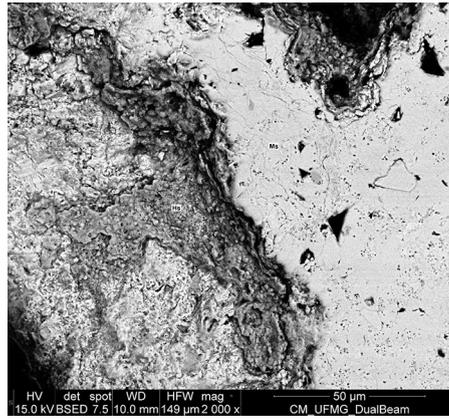
Figure 3 - Parallel bands of magnetite and hematite.
