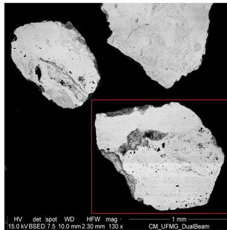
Figure 1 - Three fragments of tubercles, with approximately millimeter size.
