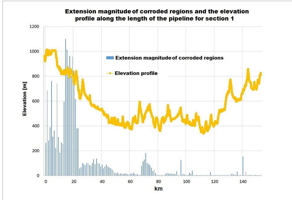
Figure 7 - Corroded regions distribution and the elevation profile along the length of the pipeline for section 1.
