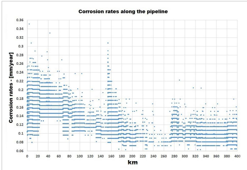
Figure 9 - Corrosion rates along the pipeline.
