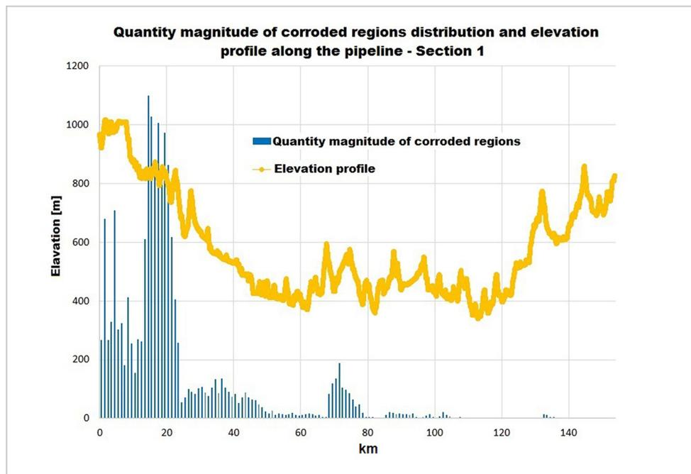
Figure 6 - Corroded regions distribution and elevation profile along the pipeline - Section 1.
