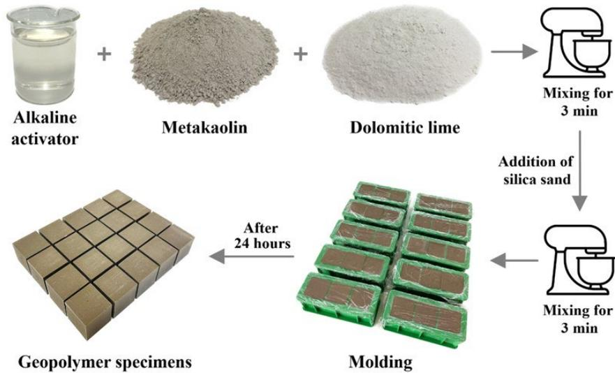
**Figure 3.** Steps in the preparation of geopolymer mixtures.
