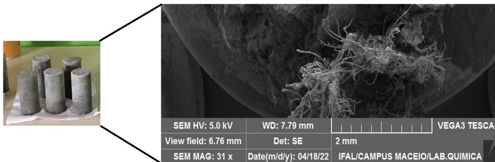
**Figure 7:** SEM image of the fractured surface of CE10 at 31 $\times$ .
