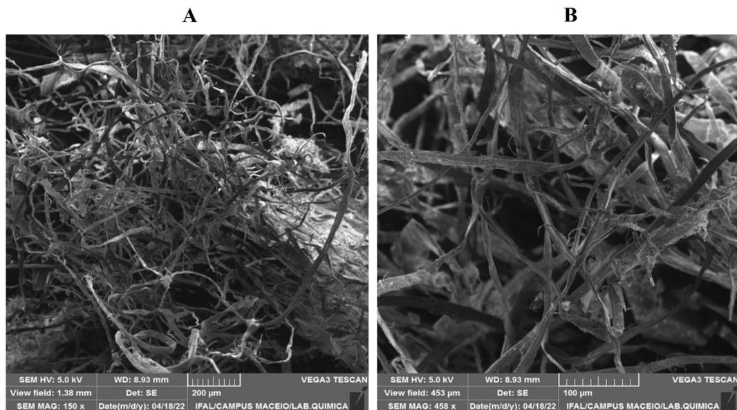
**Figure 3:** SEM of the PCPW with magnifications of 150× (A) and 458× (B).
