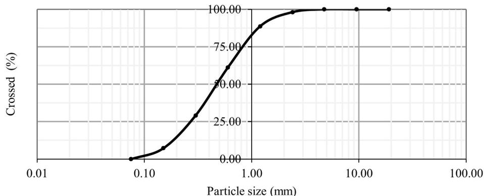
**Figure 2:** Fine aggregate granulometric curve.
