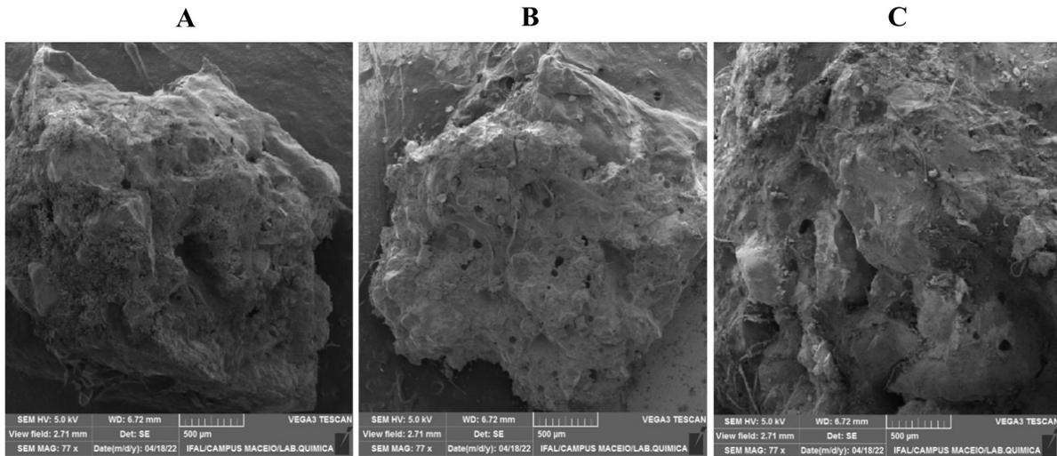
Figure 5: SEM of fracture surfaces in the cylindrical specimens of RC, EC5 and EC10.
