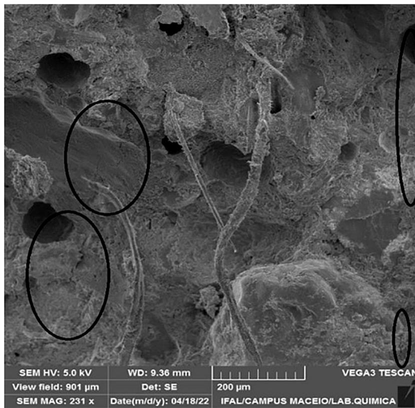
Figure 6: SEM image of the fractured surface of CE5 at  $231\times$ .
