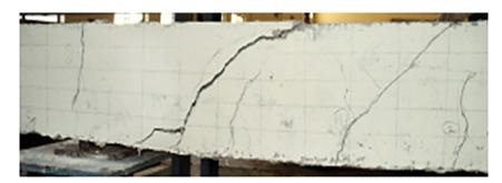
Figure 9: Pattern of beam B1a failure.
