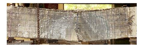
Figure 11: Pattern of beam GB1 failure.
