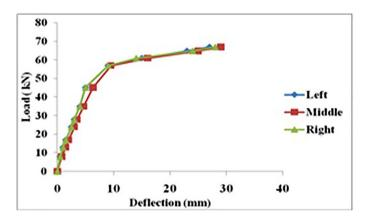
Figure 10: Curve of load versus deflection for beam GB1.
