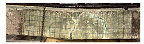
Figure 13: Pattern of beam GB2 failure.
