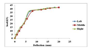
Figure 8: Curve of load versus deflection for beam B1a.
