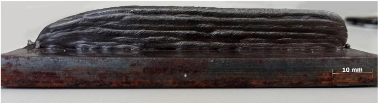
Figure 11. Wall deposited for longitudinal tensile testing samples.
