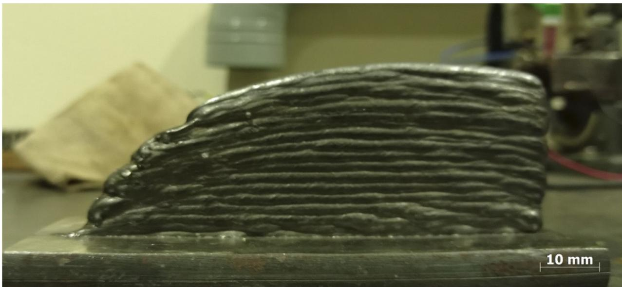
Figure 10. Wall deposited for transversal tensile testing samples.
